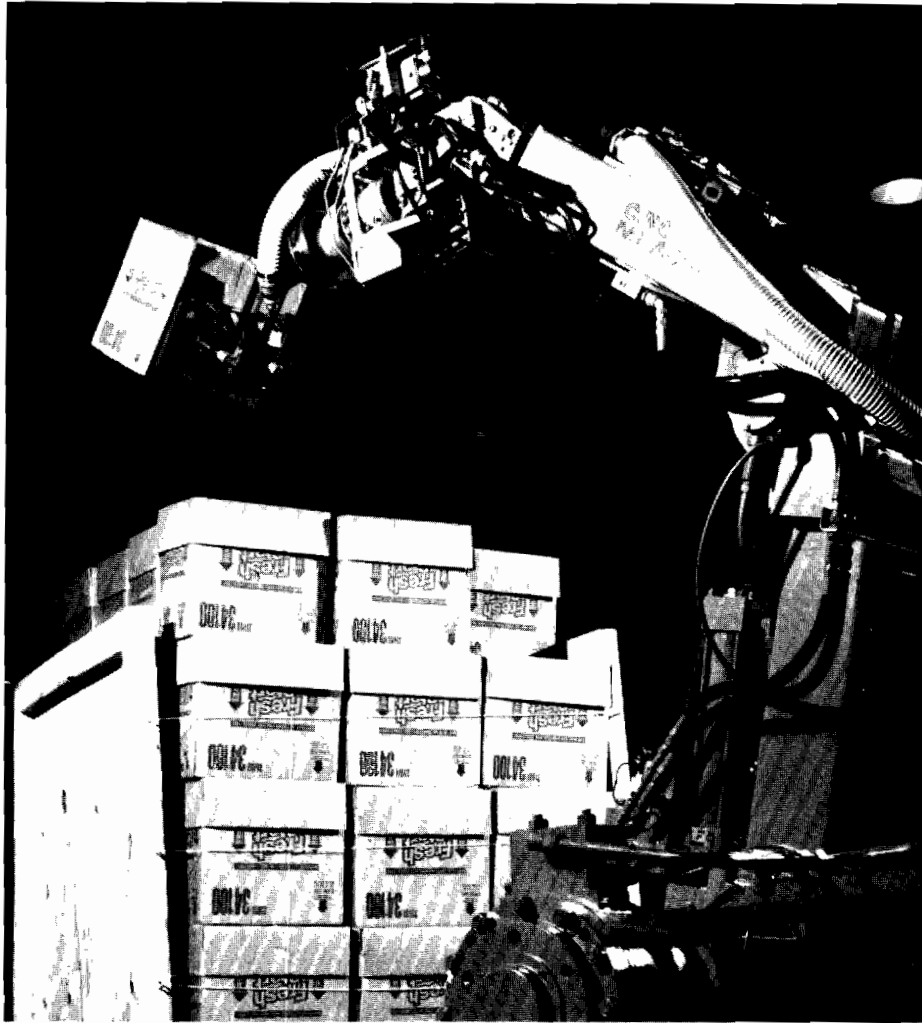
Figure 6-22. A Cincinnati Milacron HT3 robot stacking boxes in a palletizing operation. A special software function called index makes such operations easy to program. (Courtesy of Cincinnati Milacron.)
