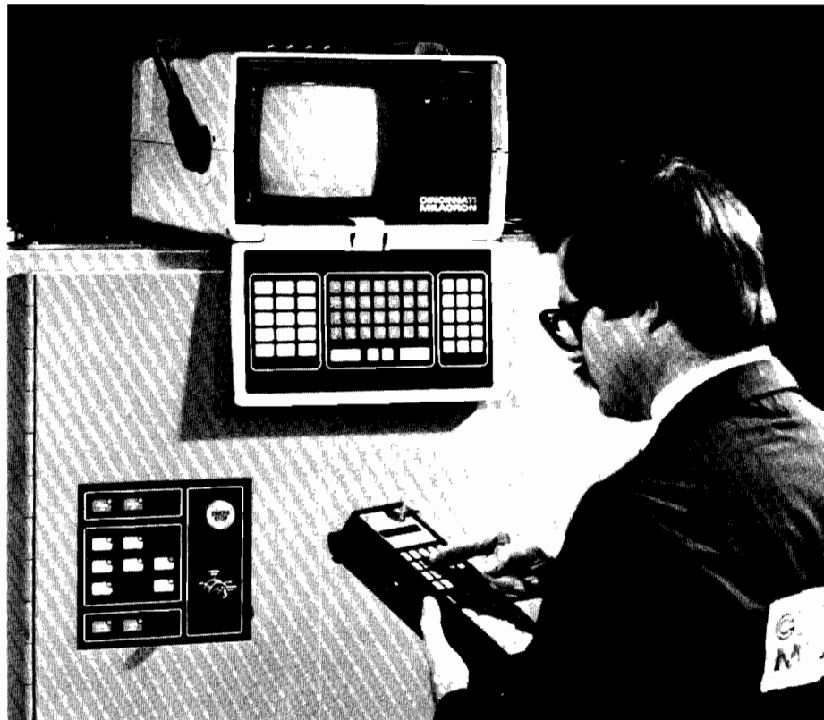
Figure 4-7. Teach pendant for the Cincinnati Milacron T3 robot. (Courtesy of Cincinnati Milacron.)
