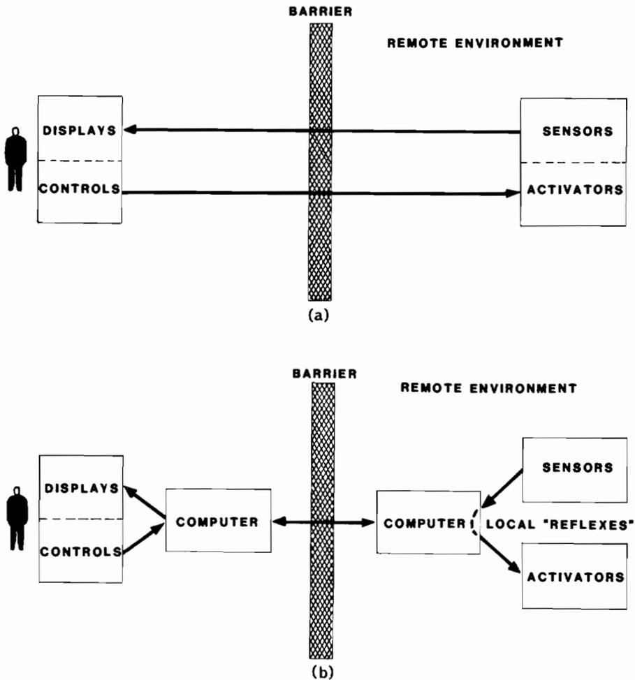
**Figure 2-3.** The basic concept of a master-slave manipulator. (a) The human, through the use of controls and displays, controls the activators and monitors the sensors in the remote environment. (b) The remote manipulator with local reflexes built into the manipulator. The use of some human control and some machine control is often required in difficult problems. (Courtesy of Microbot, Inc., Mountain View, California.)
