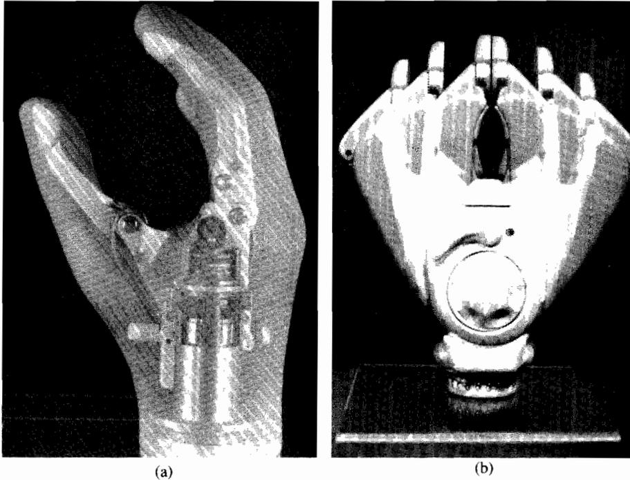
**Figure 2-1.** A modern prosthetic hand. (a) This x-ray image of the device shows the outer covering, the internal mechanical structure, and the servo motors. (b) The prosthetic hand's gripping action is shown in this multiple-exposure x-ray image. (Courtesy of Otto Bock Orthopedic Industry, Inc., Minneapolis, Minnesota.)
