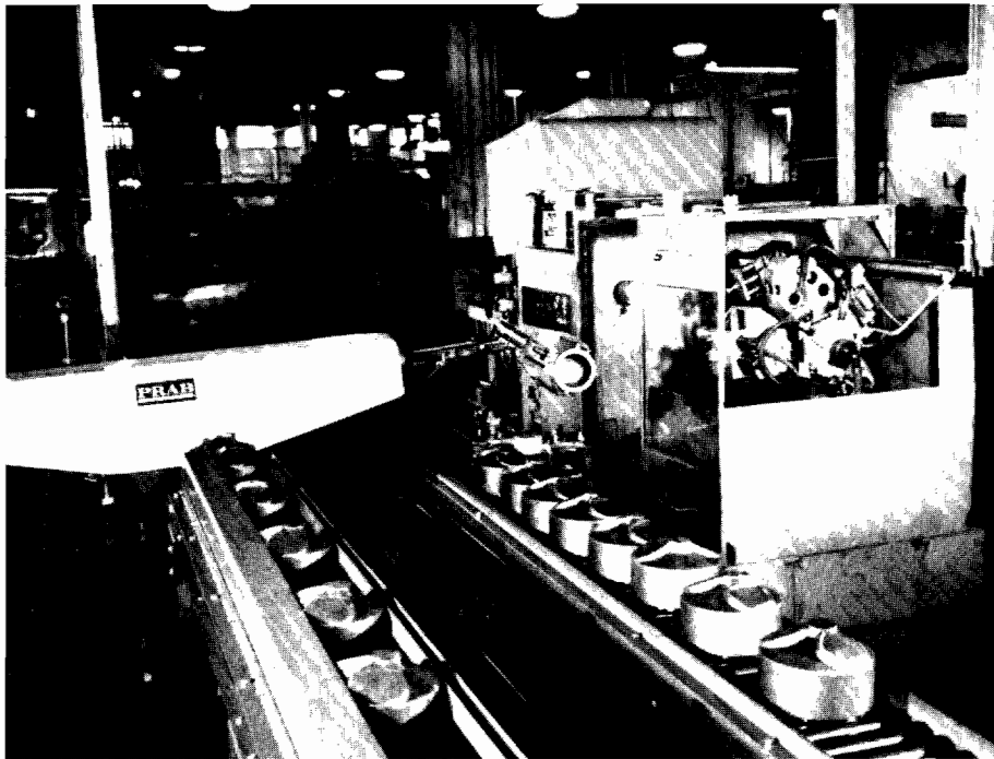
Figure 1-2. The Prab Model 5800 nonservo controlled industrial robot shown loading cylinder heads in a machining application. (Courtesy of Prab Robots, Inc., Kalamazoo, Michigan.)
